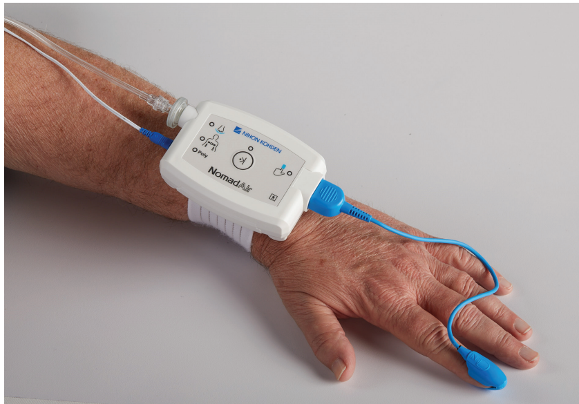
Wrist configuration records actigraphy for TST calculations. Includes pressure signal (PAP compatible), snore, SpO 2 , pulse, plethysmography signal, and RIP belt.
